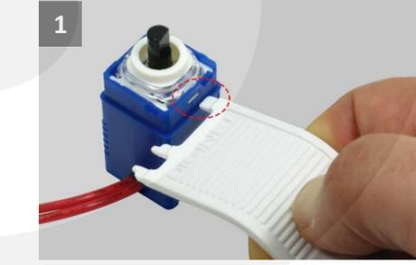
1 Use the Bezel and Dial Remove Tool (A) to engage with the slot on the side of the push button housing, as shown above.
