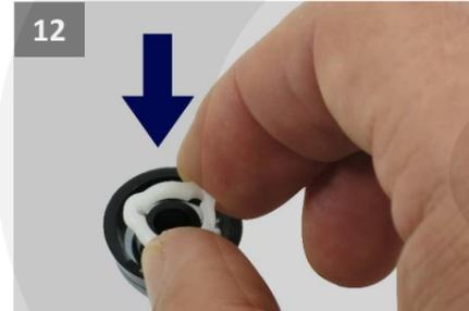
Take a Dial Clamp Ring (G) from the kit and push it firmly onto the outside of the shaft sleeve.
