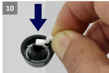
Insert the silicon Rotary Adaptor into the shaft sleeve, ensuring the vertical tab is inserted into the slot.
