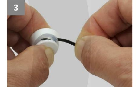
Push the cable tie along the edge of the groove, rotating the dial towards the cable-tie at the same time. Continue to push the cable-tie along the groove until the point pops through the front edge of the Dial Ring groove.
