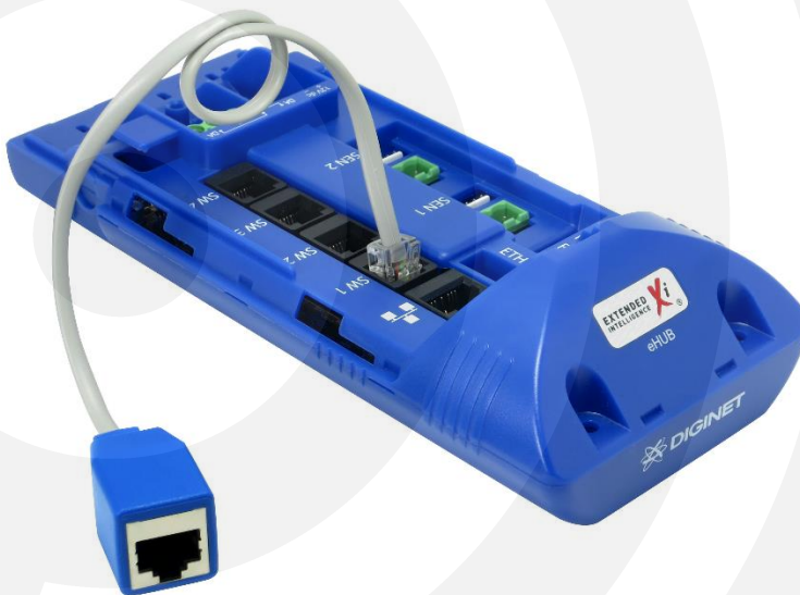
Connection between the eHub and RJ-45 patch lead
